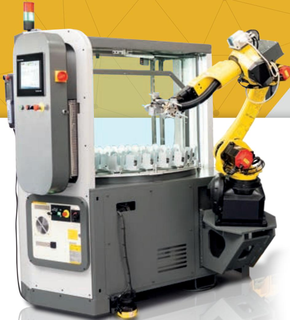
**With the Cubebox Blues RT, you can create more stock space by stacking diameter parts on top of each other and can integrate long shaft parts into the automation system.**
